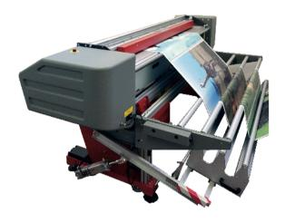
The XLD SERIES can be set in line to any printer by means of a pneumatically controlled buffer. While the printer is plotting, the buffer accumulates the media controlling the action of the cutter. It is available for all XLD cutters independently from speed and width.
