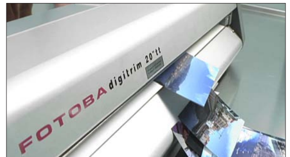
Can cut different sizes in the same roll (Digitrim nesting)
